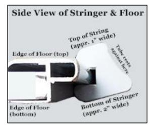
pieces. The only purpose of the stringers is to cover the joints of the aluminum panels. This is what will provide stability of the floor. This is tricky because it is a tight fit. It may help to have another person pulling up on the tubes using the straps that hold the seat.
